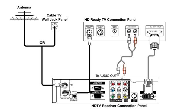
Connect the "Antenna/Cable" to the "ANT IN" jack on the HDTV Receiver using a coaxial RF cable.
